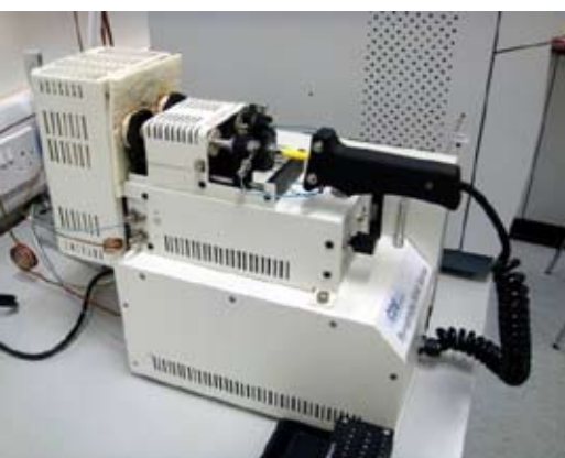
Pyrolysis-GC-MS used at Aston to screen the pyrolytic decomposition products, bio-oil and char characterisation
