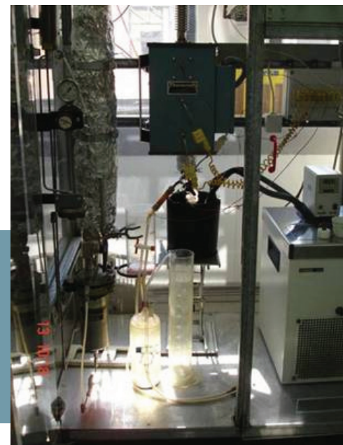
CERTH/CPERI small scale catalytic pyrolysis unit of Acid Hydrolysis Residues
