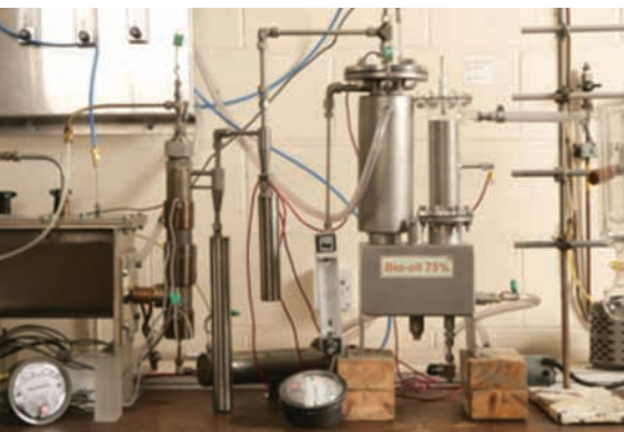
300g/hr pyrolysis unit at Aston
