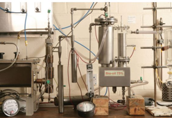
300g/hr pyrolysis unit at Aston
